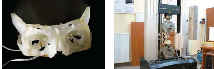
Fig. 1. The orbital model with strain gauges and in testing machine Instron 4485.
