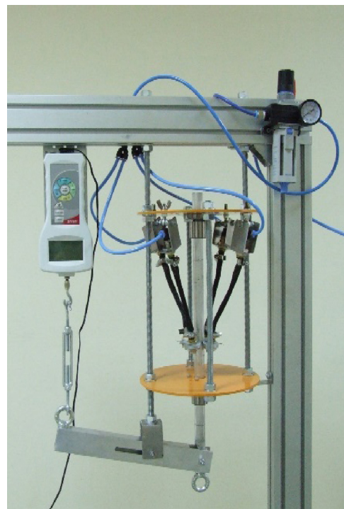
Fig. 16 – A prototype of pennate muscle (a prototype is composed of four artificial pneumatic muscles) [19].
