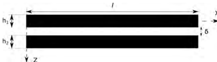
Figure 2 Scheme of beam two-layers and the temperature action ( T = 0 ).
