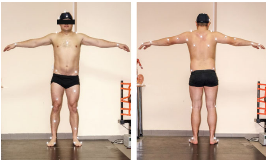
Fig. 3 Thirty seven passive reflective markers distributed on the faller’s body for observation of a forward falling process by using the Optitrack system
