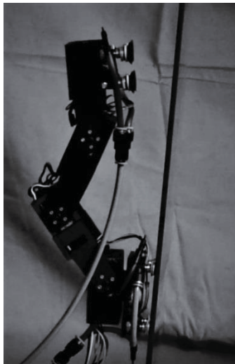
Figure 13. Climbing of inch-worm robot on the glass plate
