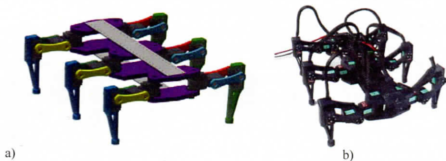
Fig. 8.3. Studied hexapod robot: a) CAD model created in Inventor, b) constructed prototype
