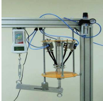
Figure 13. A prototype of pennate muscle (a prototype is composed of four artificial pneumatic muscles)
