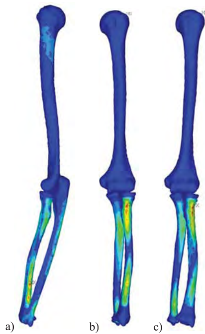
Figure 6. Maximum von Mises stress at forearm positions a) pronation, b) neutral, c) supination.
