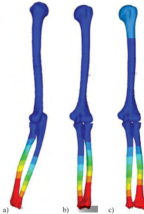
Figure 7. Maximum displacement at forearm positions a) pronation, b) neutral, c) supination.
