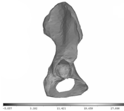
Fig. 12. 1 st principal stress for extension
