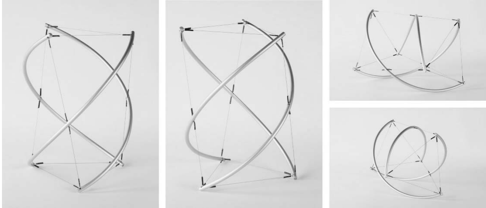
Figure 2. Manufactured model of the considered tensegrity structure in different views.
