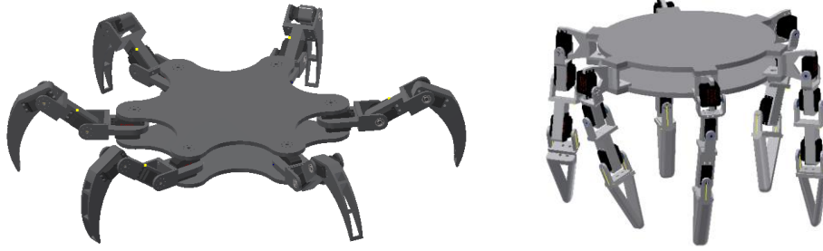
Figure 1. CAD models of bio-inspired walking robots created in Inventor Professional 2019 software: crab-like hexapod robot (on the left), and mammal-like hexapod robot (on the right).
