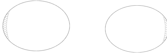
Figure 7. The domain of pure sliding in the contact surface (shaded) jumps when c changes sign
