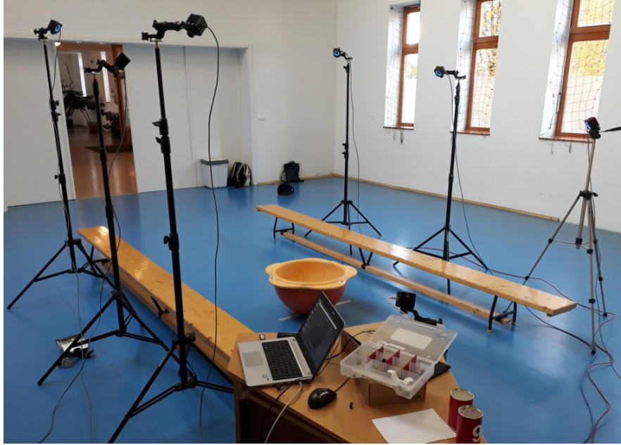
Figure 2. Experimental setup: the Huple and the motion tracking system.
