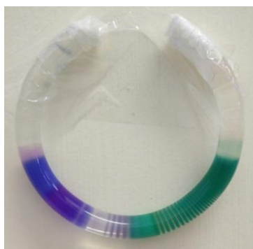
Figure 3. Complex pattern obtained by precipitation of \text{Co}(\text{OH})_2 and \text{Co}_3(\text{PO}_4)_2 in a Liesegang-type experiment carried out in a glass toroidal tube.
