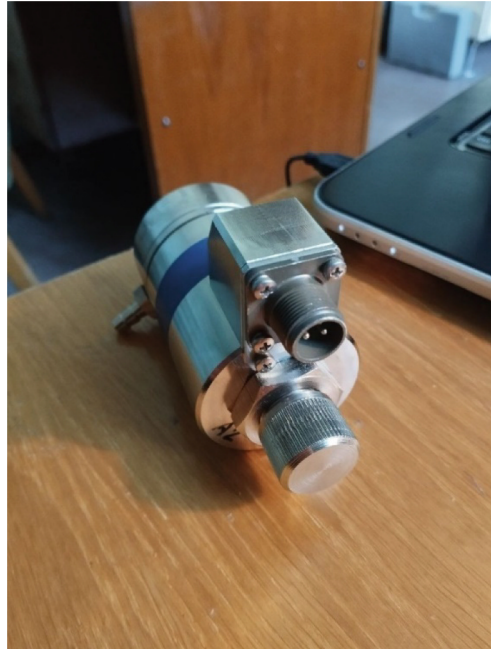
Fig. 12. Electromagnetic valve, connected to microcontroller by USB interface
