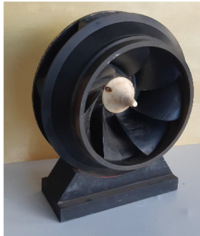
Fig. 1. Model of the R5252M7 runner (after testing on a hydrodynamic test stand).
