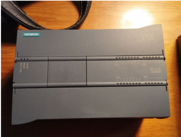
Fig. 11. SIEMENS microcontroller SIMATIC S7 1200 for ACS
